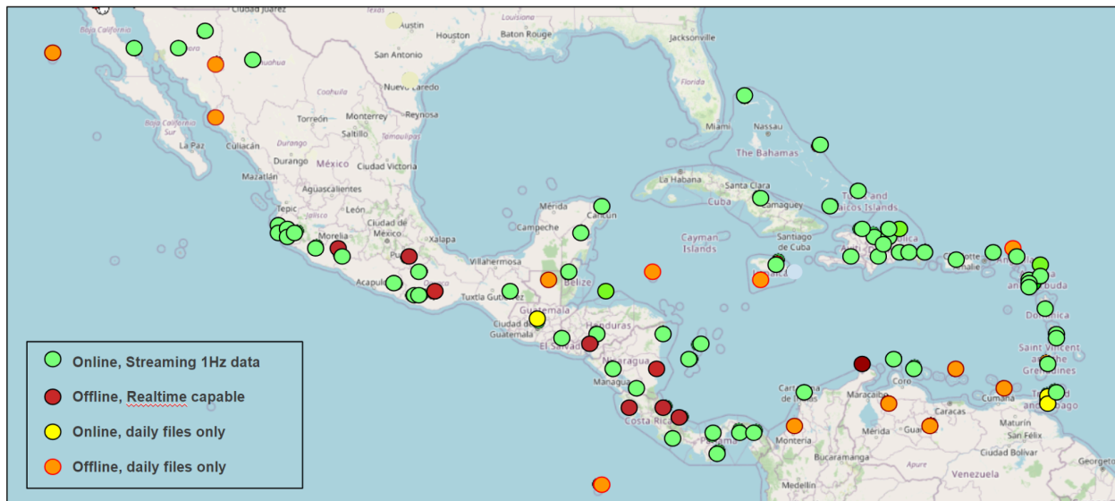
Figure 8. Caribbean regional GNSS assets within the Network of the Americas (NSF-NGF operated by the EarthScope Consortium). This includes 67 stations that are currently operational and streaming 1-Hz data which could be utilized for tsunami hazard monitoring.
