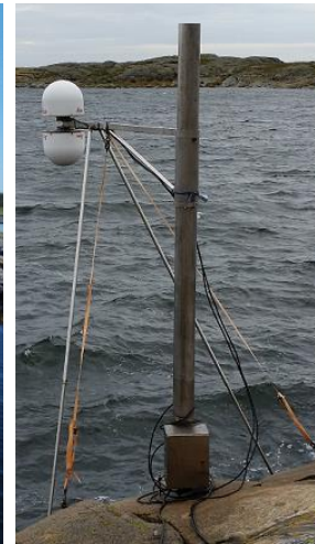
An upward- and downward looking GNSS-reflectometer.
