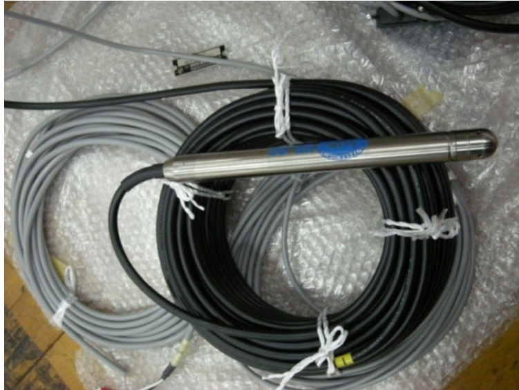
Huge Tsunami gauge using pressure sensor
