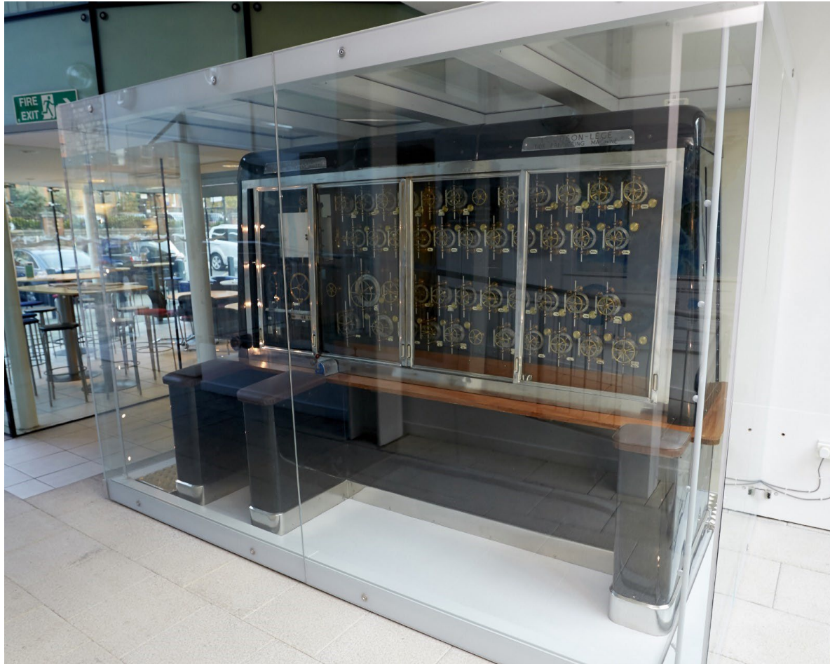
The Doodson-Légé Machine, and a close up of the mechanisms used to adjust the parameters for an individual constituent.
