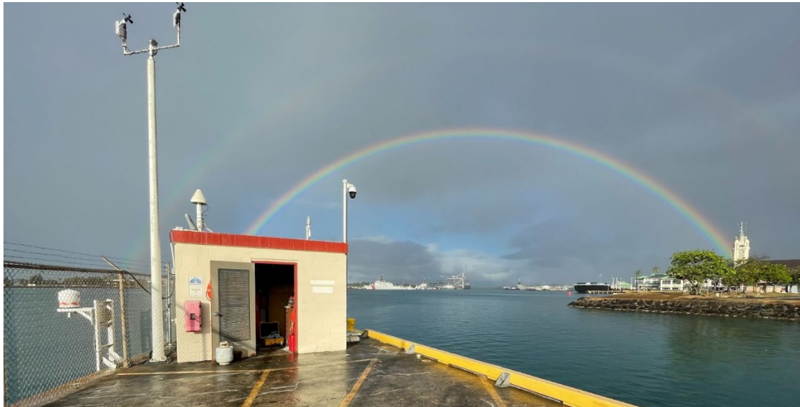
NOAA NWLON Station in Honolulu, Hawaii showing GNSS antenna, microwave and acoustic water level sensors
