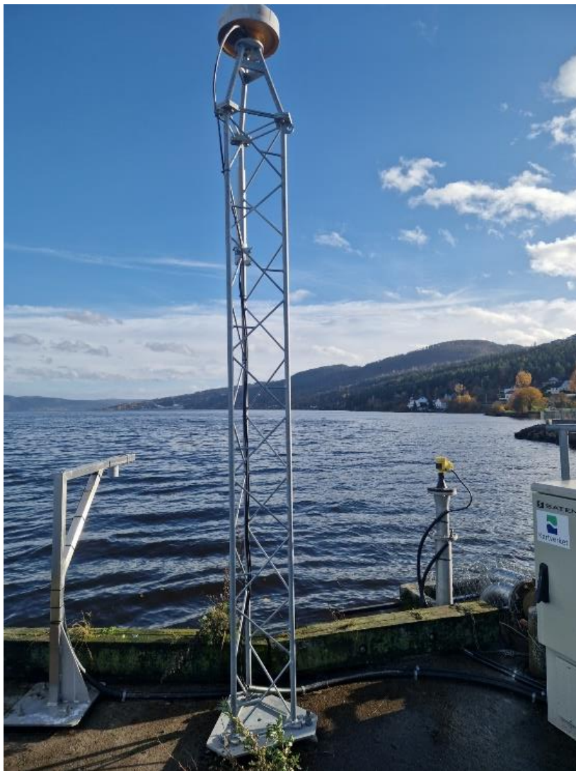
Figure 3: Tide gauge in Solumstrand
