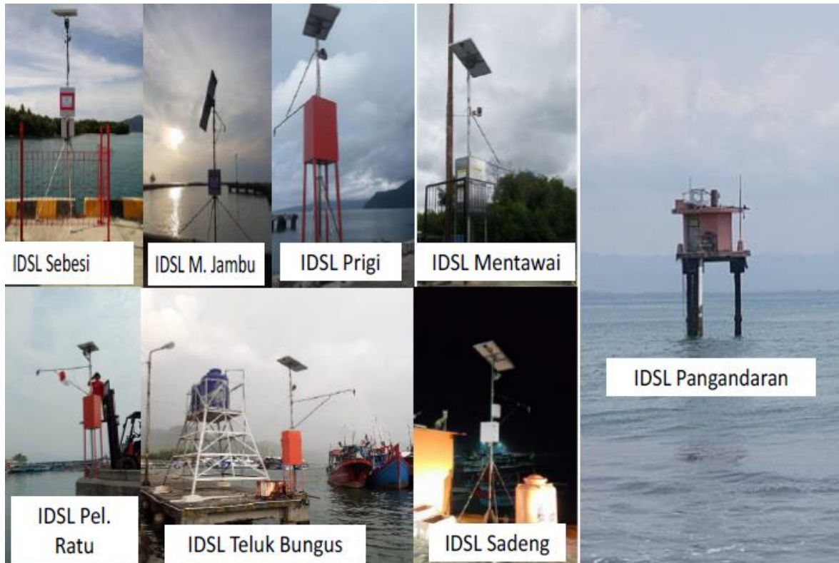
Figure 27. IDSL stations installed on the coasts of the Sunda Strait to detect tsunamis from the Anak Krakatau volcano (source: BRIN).
