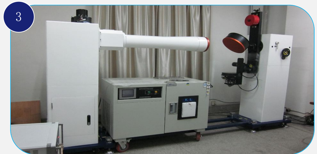
太阳模拟器及多维转台 Solar simulator and Multi-rotation platform
