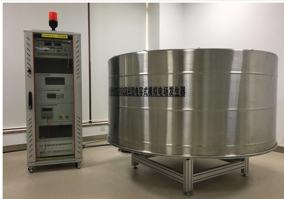
大气电场校准装置 Atmospheric electric field instrument testing device
