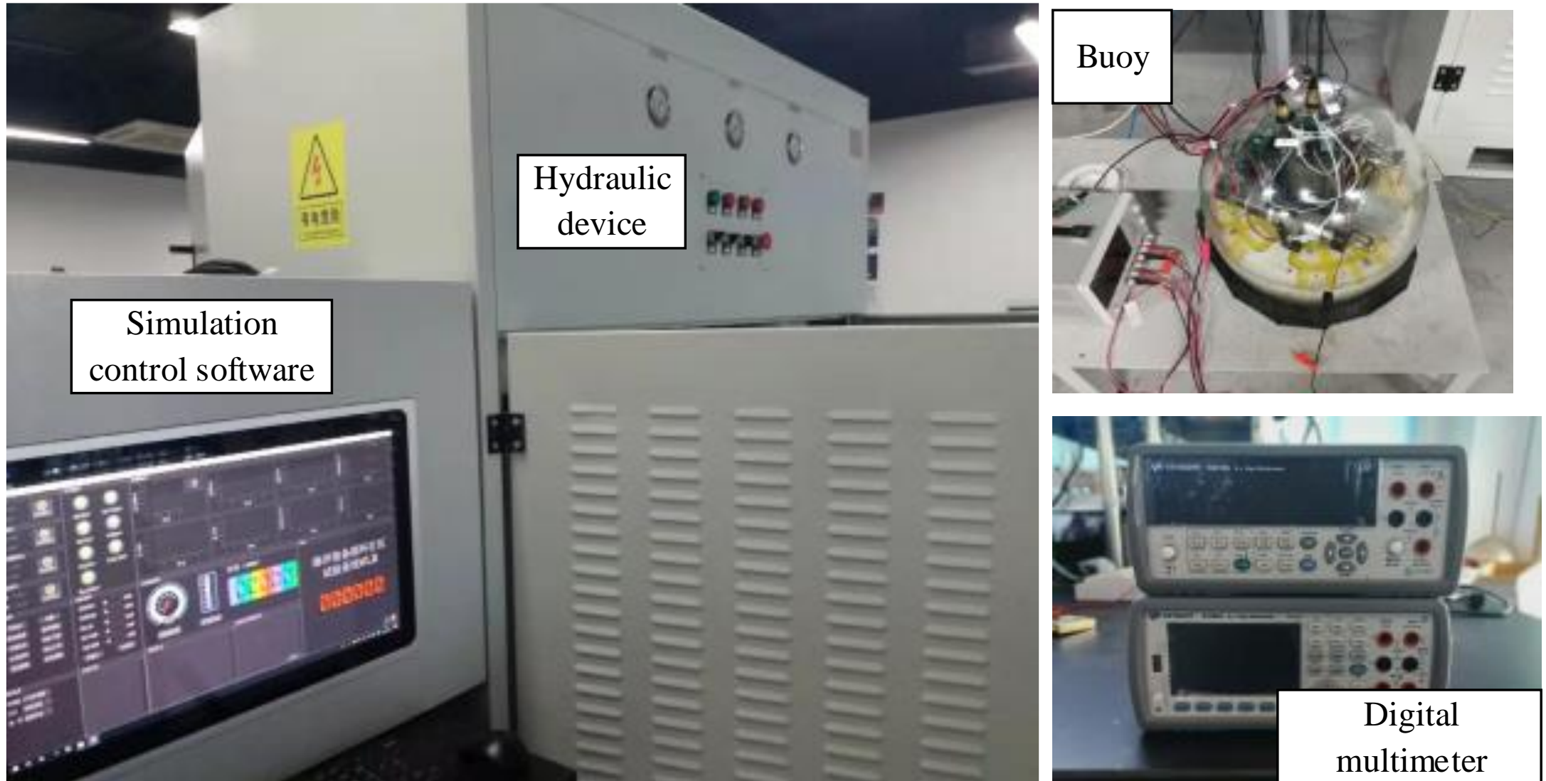
Figure 30. Hardware-in-the-loop simulation system
