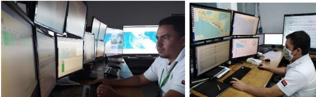
Photo 4. The seismologists of the 24x7 service perform the manual processing and must publish the results within 2 minutes after the occurrence of the earthquake.
