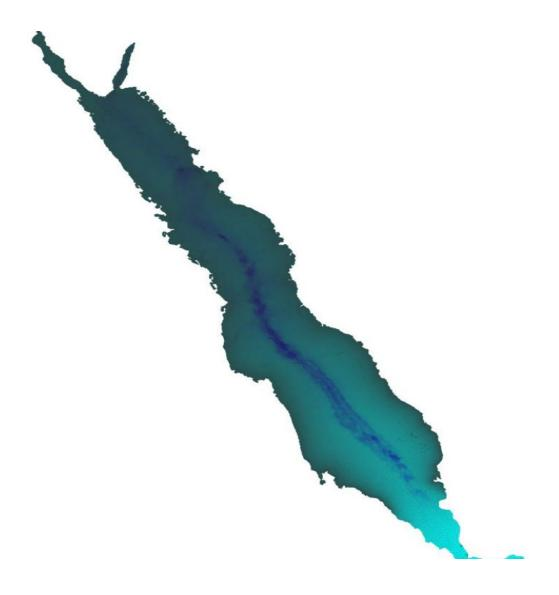
No of Nodes : 762592 No Of Elements: 1517276 Min Elevation : -2811.5 m
