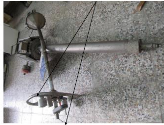
Bend of the console and sensor holder due to severe strike.
