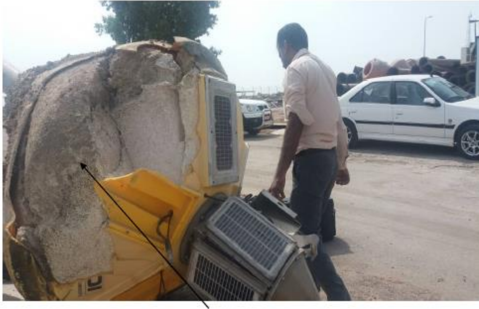
Fracture of the body of the buoy due to severe impact of a heavy object and release of the anchor
