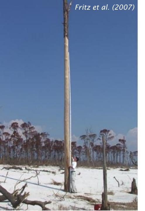
High water marks are lines found on trees and structures marking the highest elevation of the water surface following hurricane Katrina (2005)
