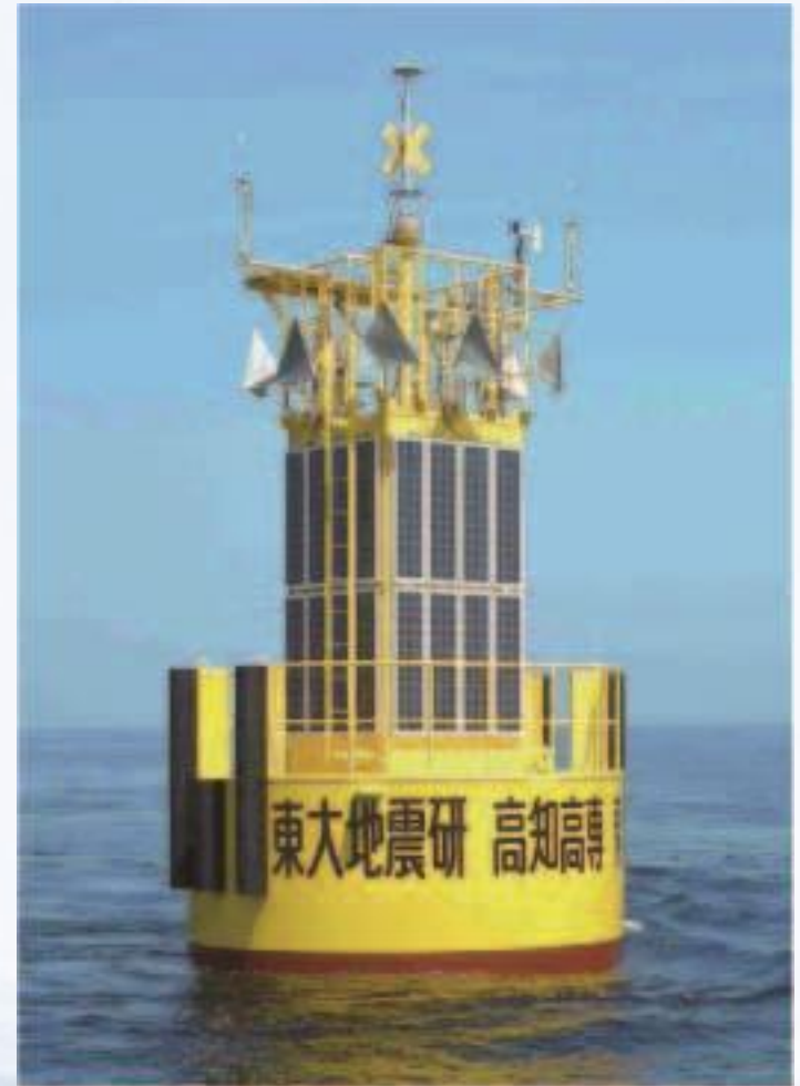
Japan GPS buoy used for tsunamis
